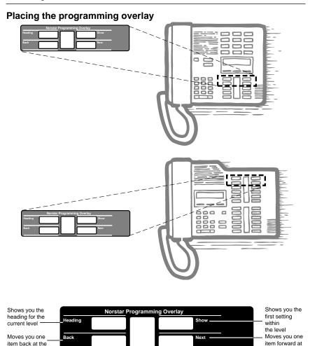
Programming buttons are active or inactive at different stages of programming. A button is active (meaning you can use that option), when the indicator next to it is lit ( $\triangleleft$  or  $\triangleright$ ).
